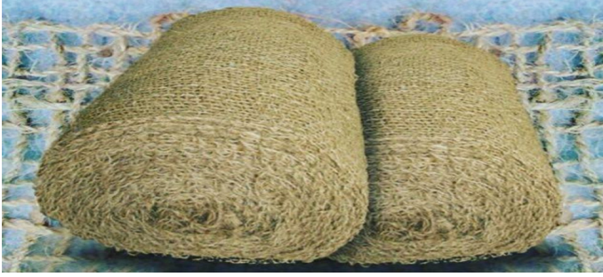
Fig. 3. A sample of natural woven geotextile made from coconut fiber
